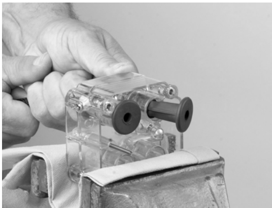
Pulling Pinch Valve through Valve Body
