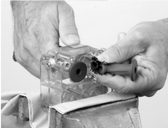
Pinching Flat Pinch Valve Up Flange
